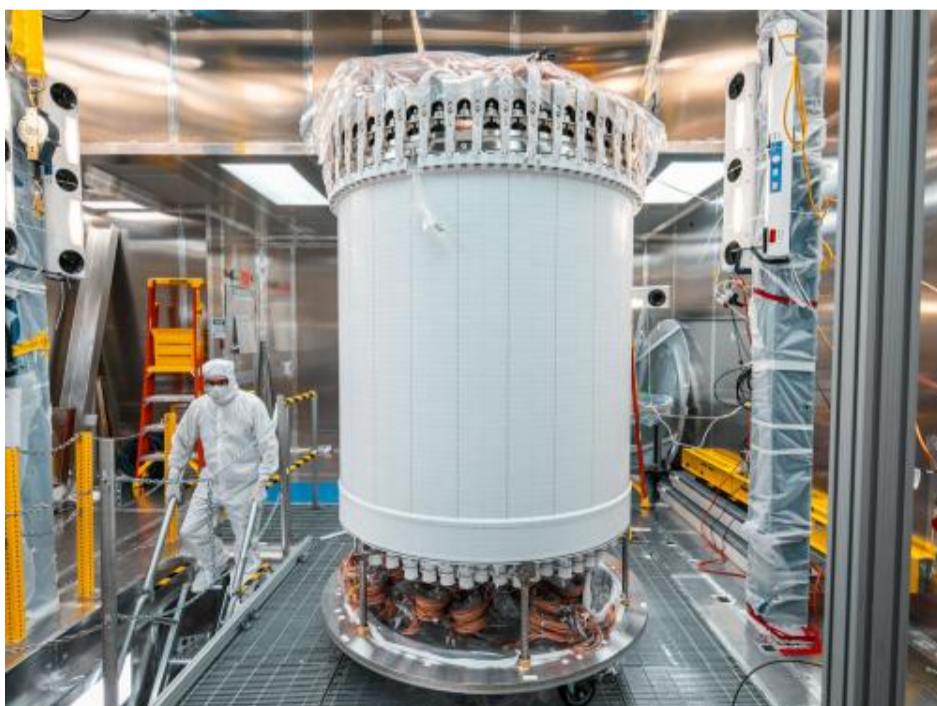
The Liquid Xenon Time Projection Chamber (TPC), the heart of the LZ detector, in the clean room before assembly inside the titanium cryostat. Credit:
